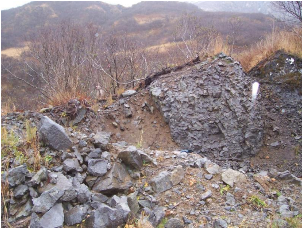
Photograph 17: Test pit excavation by landfill showing silty gravel colluvium and large blocks of volcanic rock.
